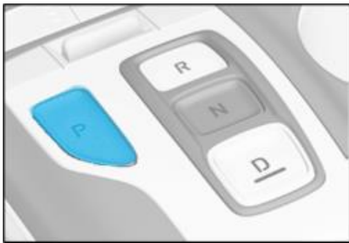
Step on brake pedal to park the vehicle, then select the shift lever in park (P)
